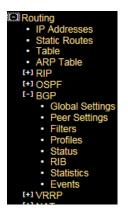
Starting with Global Settings we enable to feature, assign the AS number, and the Router ID which is simply the IP address of the Ethernet port connecting to the Verizon MPLS service.
