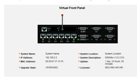
Initial Virtual Front Panel Web screen showing various system level information including software version etc.
