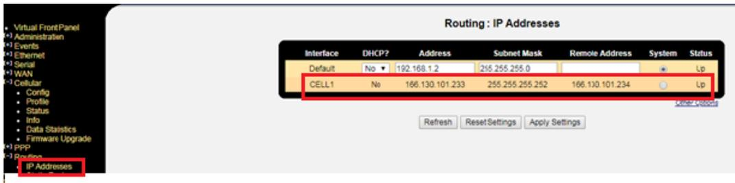
Step 7: Verify Cellular interface entry in Routing table, see picture below under **Routing àTable**
