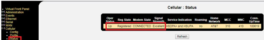
Make sure operation status is Up, Modem State: Connected, Signal Strength: Excellent
