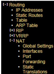
In this example we are going to select the Cell Interface, the Private Address is the address we are going to assign to the SCADA RTU, so the Ethernet ports we previously set the IP address to 192.168.2.2, so the next address .3 we will use for the RTU. We then have to select the Protocol type, either TCP or UDP, and then the associated Port numbers used in the SCADA application.
