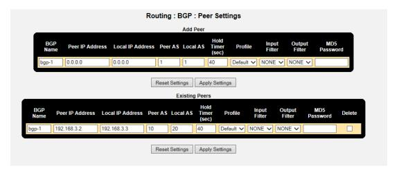
Modify the "default" profile next, here we have selected "Redist Static and BGP", this just means we will share information of local IP addresses into the BGP protocol and also learnt IP addresses through BGP placed into the routing table.
