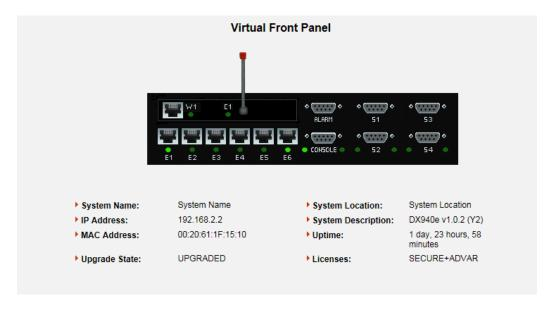
Initial Virtual Front Panel Web screen showing various system level information including software version etc.
