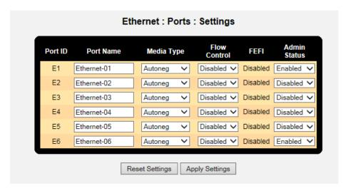
Also by default all Ethernet ports are bridged and only holds one IP address. In this case we are routing between the Control center and Verizon MPLS network with 2 different subnets, so we need un-bridge at least one port to form 2 subnets.
