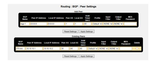
Modify the "default" profile next, here we have selected "Redist Static and BGP", this just means we will share information of local IP addresses into the BGP protocol and also learnt IP addresses through BGP placed into the routing table.
