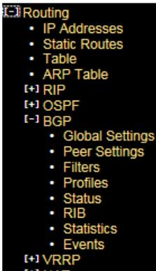
Starting with Global Settings we enable to feature, assign the AS number, and the Router ID which is simply the IP address of the Ethernet port connecting to the Verizon MPLS service.
