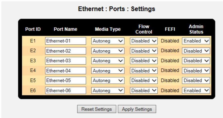
Also by default all Ethernet ports are bridged and only holds one IP address. In this case we are routing between the Control center and Verizon MPLS network with 2 different subnets, so we need un-bridge at least one port to form 2 subnets.
