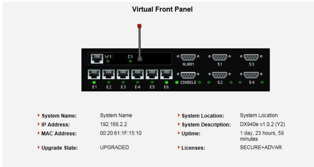
Initial Virtual Front Panel Web screen showing various system level information including software version etc.
