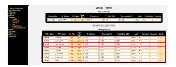
You can select one of the existing profiles, if the profile with APN name is not in the list, you can create one based on Profile parameters provided by Verizon Service Provider. Click on Apply settings.
