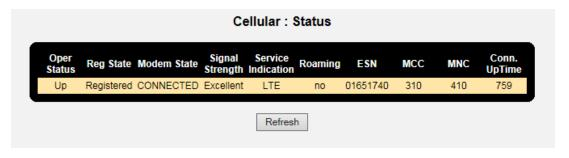
In the above example, the cellular interface is connected to the network, and the Operation Status is Up. The signal strength is **Excellent**, as the signal strength indicator displays.
