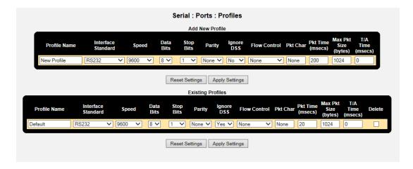
We can check the status, the Ignore DSS parameter enables the port rather than needing additional signals like DTR from the RTU.
