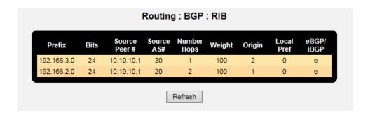
Finally a look at the full IP routing table to check we have full connectivity of the network
